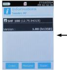
The probe information is displayed With the function key "Meas." It is possible to back to the measurement screen. It is also possible to delete the wireless probe pressing the function key "Delete".
